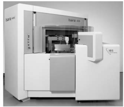
Fig. 2 Photograph of the Isara 400 CMM
